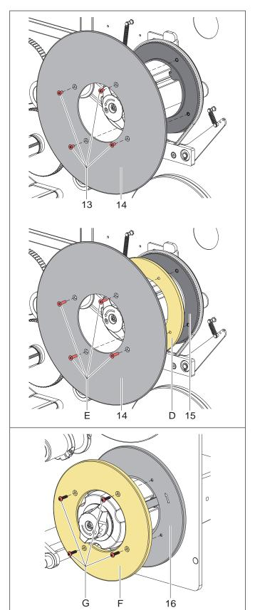
Mounting the Distance Washer at the Label Unwinder
